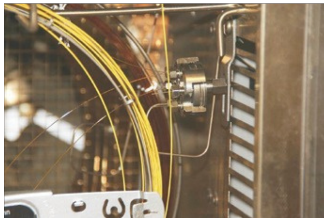
Figure 2. Photograph of installed system showing the S-Swafer connections.
